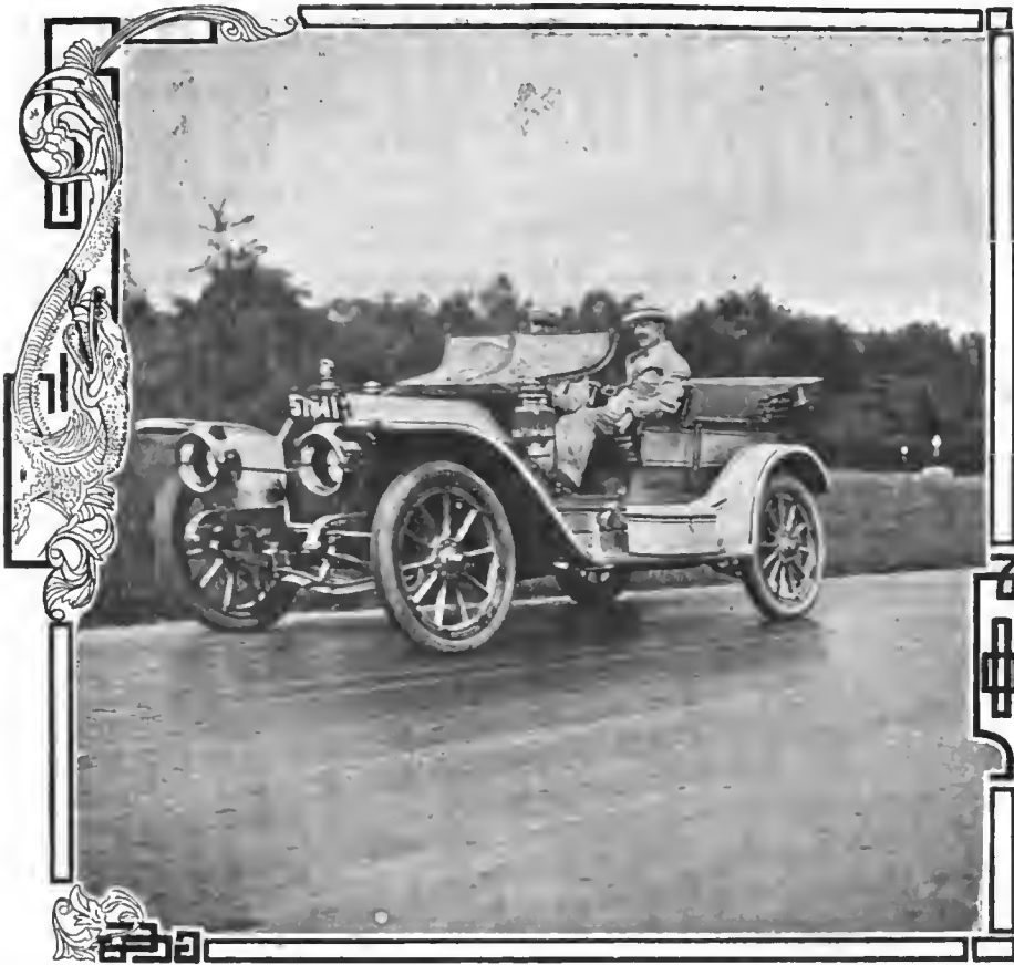
C—Showing a powerful touring car traveling over the cement brick surface at a fair speed without the slightest sign of dust
